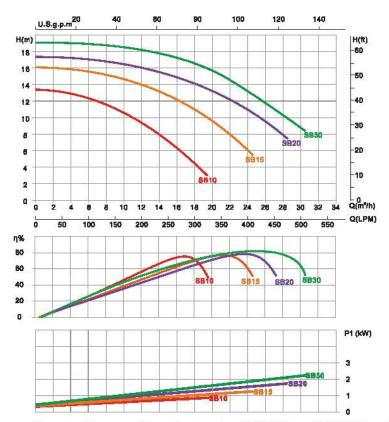
Remarks: Flow curve information based on 220V/50Hz and 380V/50Hz motor.
